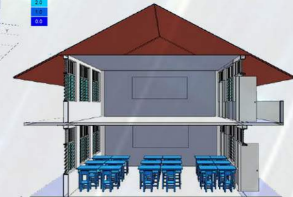
Current JKR Classroom Walls on all four sides (lack of thermal displacement)
